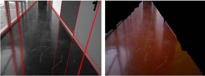
Fig. 8. Example of the polygonal-based segmentation algorithm. Left image shows the extracted lines forming the polygonal regions. Right image shows the corresponding polygonal-based floor segmentation.
