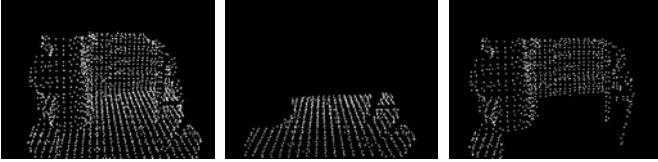
Fig. 3. Left image shows the filtered point-cloud. Center and right images show the first detected plane and the point-cloud after first plane extraction, respectively. This last point-cloud will be processed again in order to extract the next plane of the scene, and so on.
